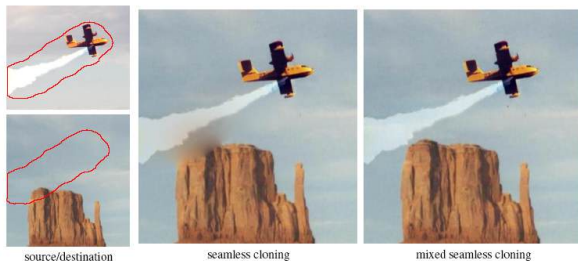
Figure 8: Inserting one object close to another. With seamless cloning, an object in the destination image touching the selected region \Omega bleeds into it. Bleeding is inhibited by using mixed gradients as the guidance field.
