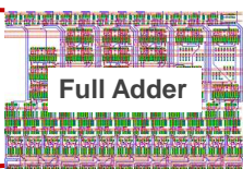
Register Transfer Level (RTL) Design 1K~10K Cells/Module (100K Devices)
